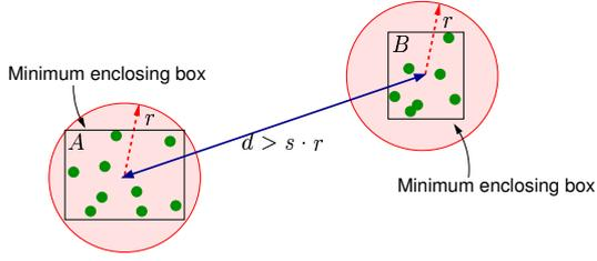
Fig. 5. Clusters  $A$  and  $B$  are 'well-separated' if  $d > s \cdot r$ .
