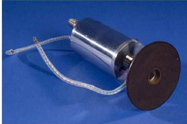
Slika 2. Maimanov laser Izvor: Izložba Fifty Years Of Lasers, National Museum of American History, Washington, DC
